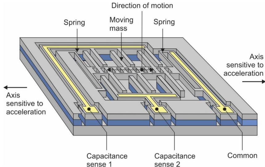
**Figure 1. MEMS accelerometer die.**
