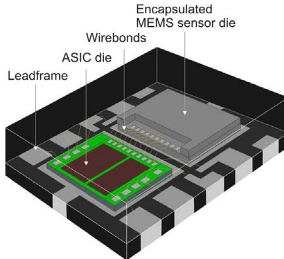
**Figure 2. MEMS accelerometer and IC die packaged together as a MEMS product.**
